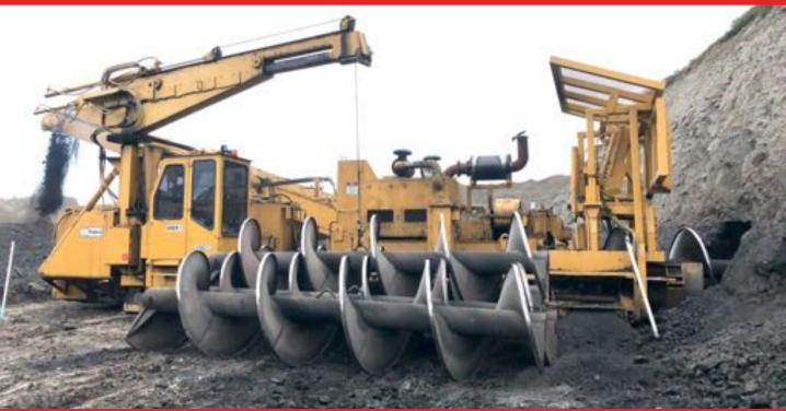
**AUGER MINING** is a surface mining technique used to recover additional coal from the exposed coal seam at stripping limit.
